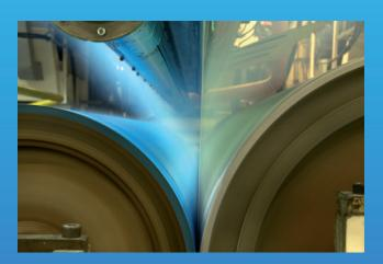
Hot-Melt lamination: one or more layers of Nowoven are laminated with the microembossed antimicrobial polyolefinic film by UFD technology (Uniform Fibres Deposition). Thanks to UFD technology, these laminates have outstanding drapability, softness and absorption rate.
